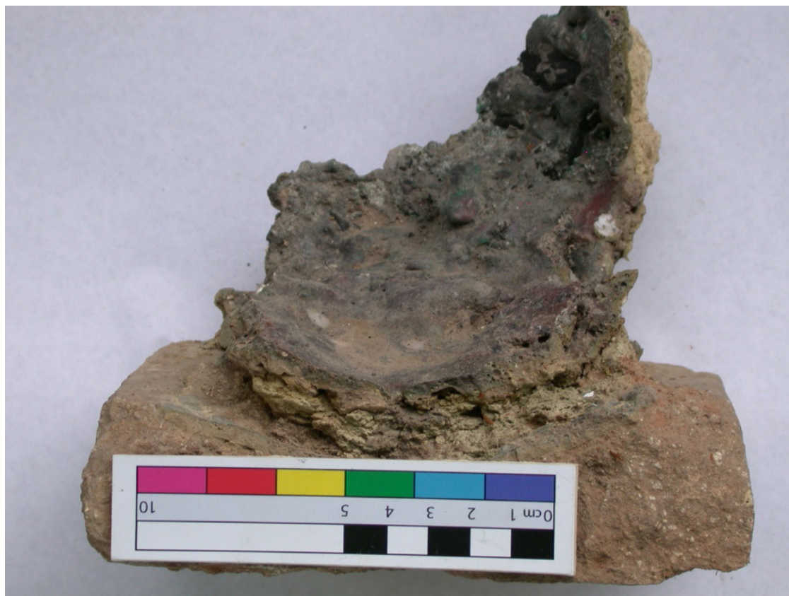
Figure 3a. Small copper furnace, built on a tile for support. Akhsiket Excavation Magazine.
